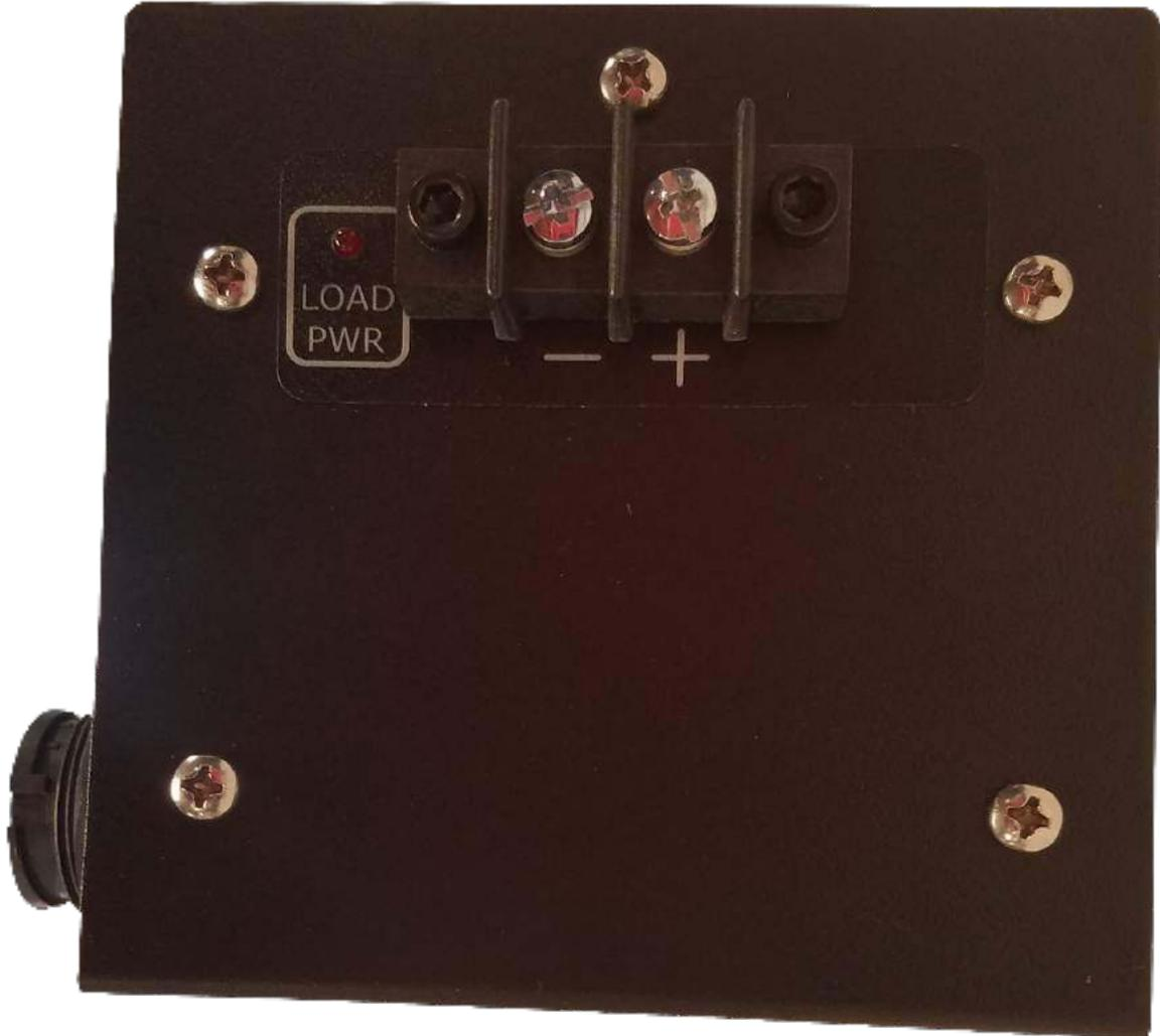
Recommended wire size for +12V and GND to the CDRV-HI is 14-16 gauge wire.
